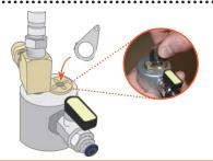
Replace the brass valve plug and tighten until hand-tight. DO NOT over tighten.
