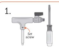
Loosen the set screw with flat head screwdriver.
