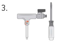
Re-tighten the set screw. Avoid overtightening and stripping the screw.
