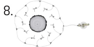
Lay the Q-connect harness around the base of the tree. Ensure both ends of the harness are connected (connector should "click") and the harness is connected to the bottle.
