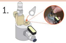
Use a coin or bottle top key (Field Repair Kit) to unscrew the brass valve plug.
