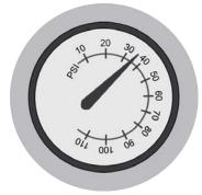
Pressurize the bottle to 35 psi. If more pressure is needed, the bottle can be pressurized up to 55 psi.
