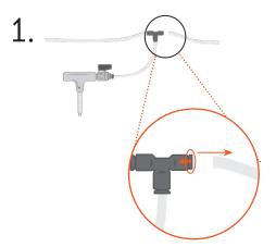
Remove tubing by pushing in and holding the collet, then pulling out the tubing.
