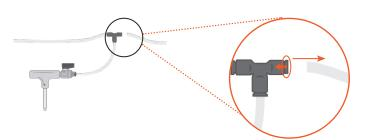
To disconnect tubing, push in the plastic collet of the push-to-connect and pull out the tubing.
