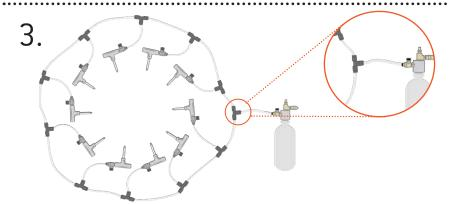
If the connector stops functioning in the field, remove the harness connector and connect both sides of the harness to a black push-to-connect tee that will feed directly from the bottle to finish the work. Clean or replace the harness connector.
