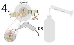
With the main bottle valve closed, unscrew the bottle top and pour the measured product dose into the bottle, OR use the Q-gun or iQ-infuser to dose the bottle directly through the dosing port.
