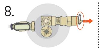
Slowly and carefully use the pressure relief valve on the bottle cap to depressurize the bottle.
