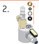
Remove the rubber grommet, metal shim, and retaining ring.
