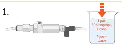
If harness connector is not connecting or is leaking, disconnect from tubing and clean thoroughly with a mixture of isopropyl alcohol and water.
