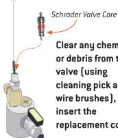
Clear any chemical or debris from the valve (using cleaning pick and wire brushes), and
