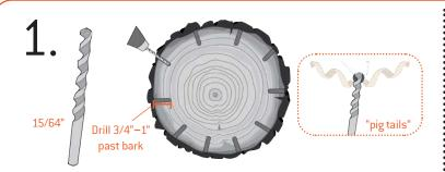
Drill injection holes using a 15/64" high helix drill bit. Drill into the root flares, 3/4"- 1" past the bark, and perpendicular to the bark surface.
