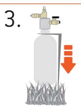
Insert the bottle stand into the ground to support the bottle.
