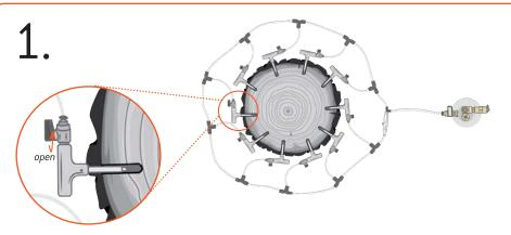
Open the valve on the tee farthest from the bottle.
