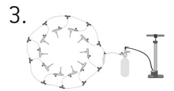
Screw on the bottle cap. With the harness connected and the injection tee valves closed, pressurize the bottle with a bike pump to 40 psi.
